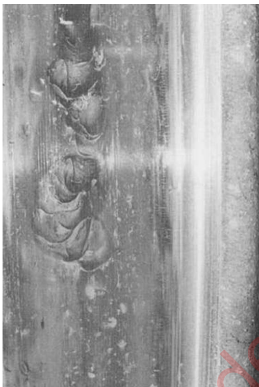
Figure 7:1 – Class 3 skidded wheel (multiple class 2 skids)
