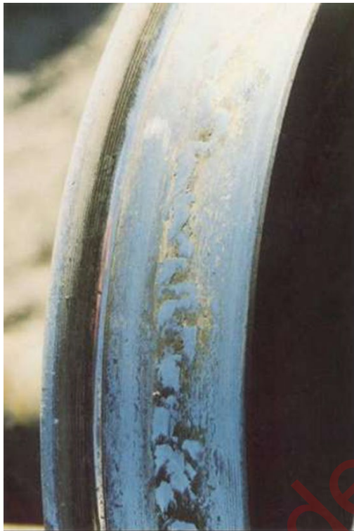
Figure 8:1 – Class 3 Scaled wheel
