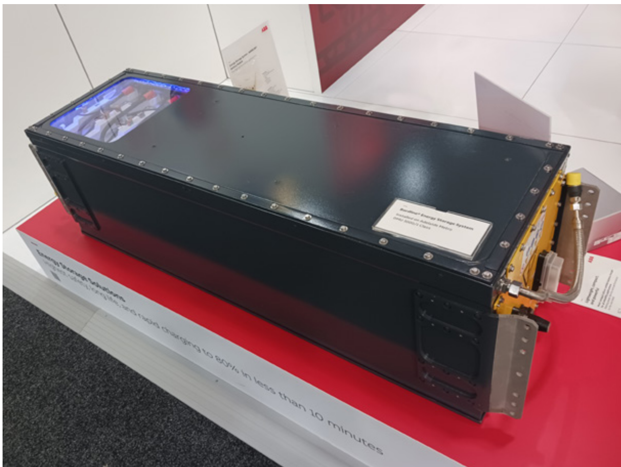
Figure 1: ABB Battery Module for 3000/3100 Class DMU
