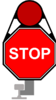
Appendix Figure C-5 Example track work stop sign
